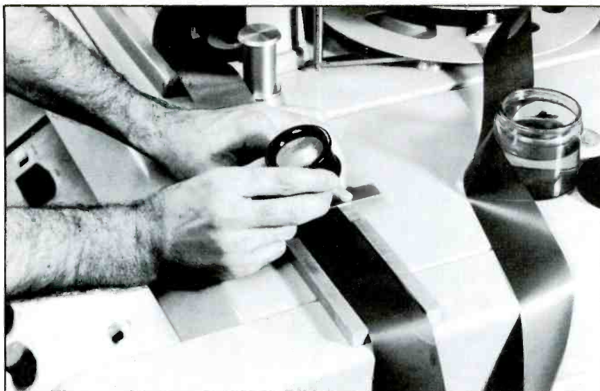
The first VTRs had no electronic editing capability. Here, an engineer prepares to physically cut the tape to effect a splice.
