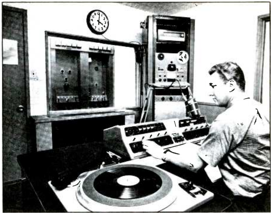
The turntable and reel-to-reel tape recorder were primary sources for radio programming in 1955. Modern radio stations seldom rely on reel-to-reel tape recorders, and digital CDs provide much of the high-quality music used by many stations.
